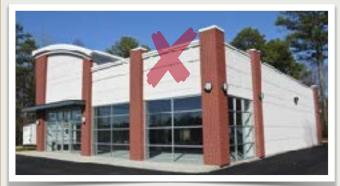
Brick Pilasters should not extend beyond the overall parapet plane. Proper balance and symmetry would require the columns to support a brick entablature with historic detailing.
