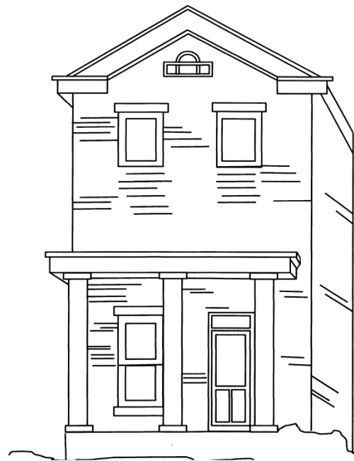
Inappropriately blocked-up windows.
